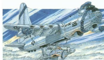
"Thunderflushed" B-36 Peacemaker modified to carry RF-84F Thunderflash
